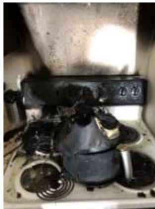
Picture of air-fryer that caused the apartment fire
