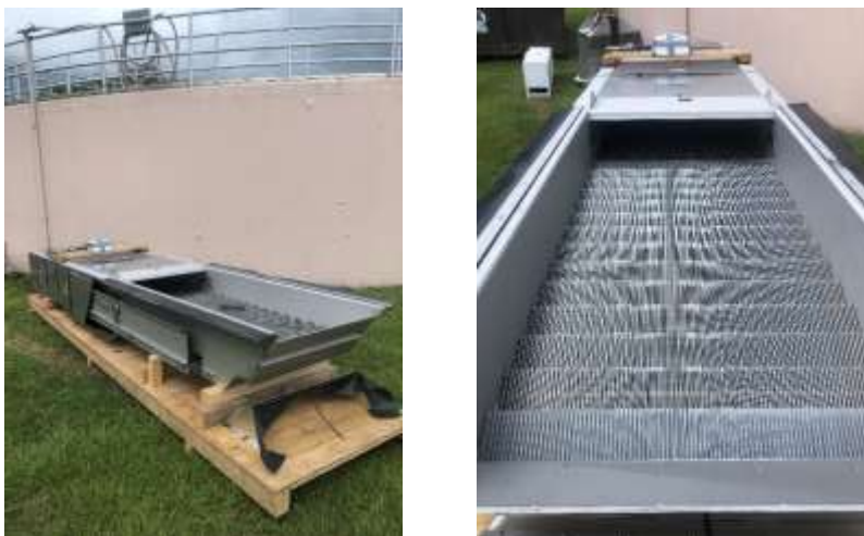
Photo of new barscreen awaiting installation at the WRF
