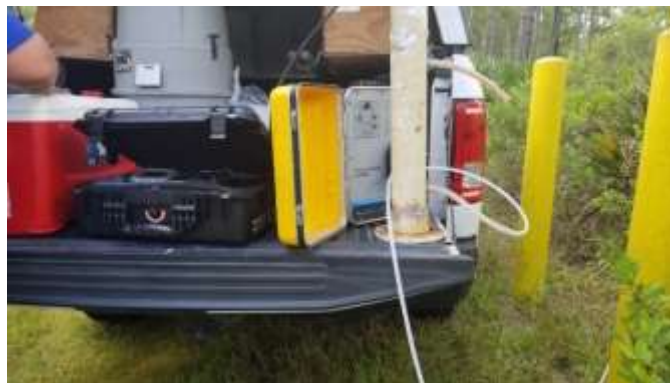
Photo of sampling equipment used to sample City groundwater monitoring wells
